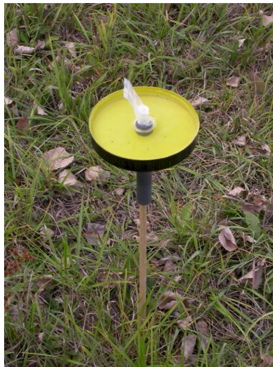
Figure 5.2.1. Water trap used in the plant volatile experiments
